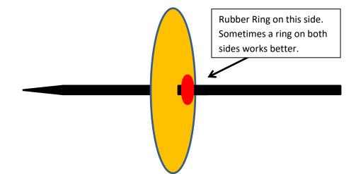
Keep a couple of made up spotters for instant use when they get a shot through them. Repair holes in the spotter immediately after they occur!! Save the repaired spotter as a spare. Two styles of pegs are supplied. Choose which works for you.
